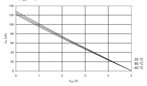
**Figure 6-153.** Atmel ATmega48PA: Reset Pull-up Resistor Current vs. Reset Pin Voltage ( $V_{CC} = 1.8V$ )
