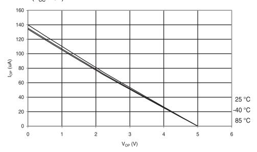
Figure 6-245. Atmel ATmega168PA: Reset Pull-up Resistor Current vs. Reset Pin Voltage  $(V_{CC}=1.8V)$
