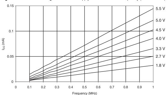
Figure 6-317. Atmel ATmega328P: Reset Supply Current vs. Low Frequency (0.1 - 1.0MHz)
