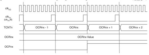
Figure 6-38 shows the setting of OCF0A and the clearing of TCNT0 in CTC mode and fast PWM mode where OCR0A is TOP.
