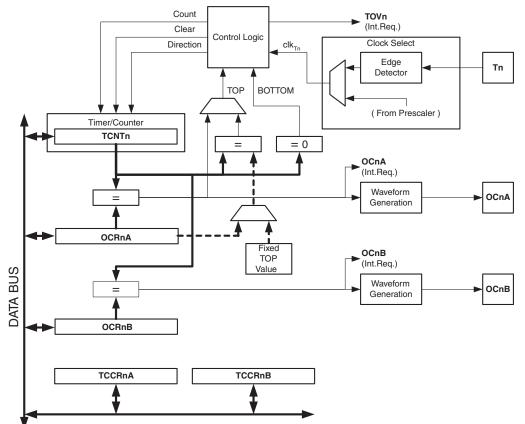
Figure 6-28. 8-bit Timer/Counter Block Diagram
