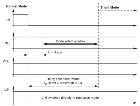
Figure 3-3. Switch to Silent Mode
