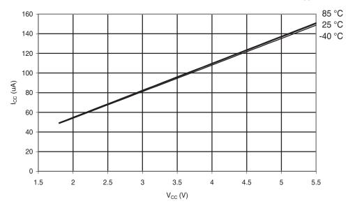
Figure 6-223. Atmel ATmega88PA: Brownout Detector Current vs.  $V_{\rm CC}$
