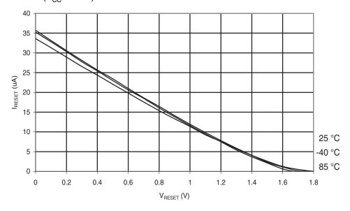
**Figure 6-246.** Atmel® ATmega168PA: Reset Pull-up Resistor Current vs. Reset Pin Voltage  $(V_{CC} = 2.7V)$
