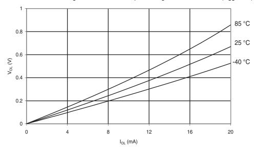
Figure 6-203. Atmel ATmega88PA: I/O Pin Output Voltage vs. Sink Current ( $V_{CC} = 5V$ )
