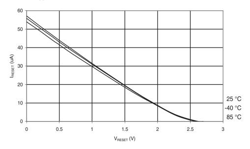
Figure 6-201. Atmel ATmega88PA: Reset Pull-up Resistor Current vs. Reset Pin Voltage  $(V_{CC}=5V)$
