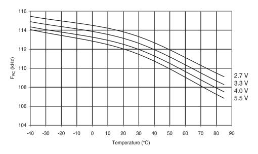
Figure 6-170. Atmel® ATmega48PA: Watchdog Oscillator Frequency vs. V<sub>CC</sub>
