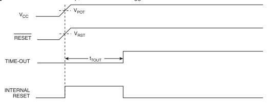
Figure 6-17. MCU Start-up, RESET Extended Externally
