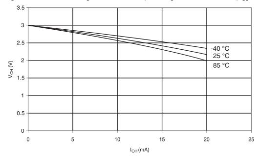
Figure 6-297. Atmel ATmega328P: I/O Pin Output Voltage vs. Source Current(V<sub>CC</sub> = 5V)
