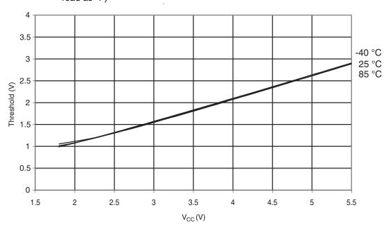
**Figure 6-299.** Atmel ATmega328P: I/O Pin Input Threshold Voltage vs.  $V_{CC}$  ( $V_{IL}$ , I/O Pin read as '0')
