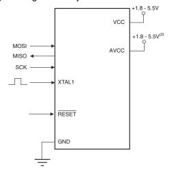
If the device is clocked by the internal Oscillator, it is no need to connect a clock source to the XTAL1 pin.
