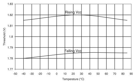
Figure 6-213. Atmel ATmega88PA: BOD Thresholds vs. Temperature (BODLEVEL is 2.7V)
