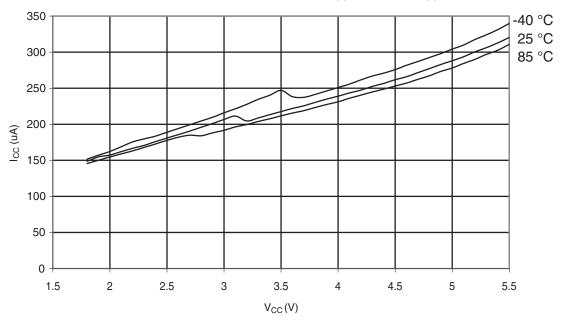
Figure 6-313. Atmel ATmega328P: Analog Comparator Current vs.  $V_{\rm CC}$
