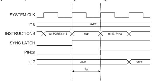
Figure 6-26. Synchronization when Reading a Software Assigned Pin Value
