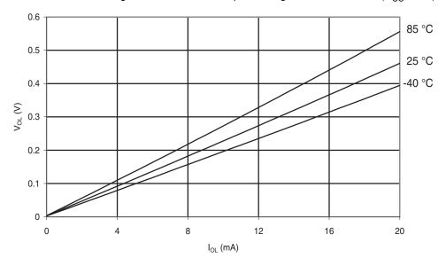
**Figure 6-250.** Atmel® ATmega168PA: I/O Pin Output Voltage vs. Source  $Current(V_{CC} = 3V)$
