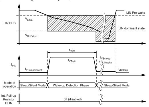
Figure 3-7. Floating LIN-bus During Sleep or Silent Mode
