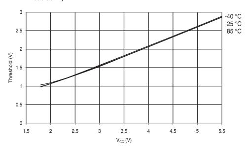
**Figure 6-161.** Atmel ATmega48PA: I/O Pin Input Threshold Voltage vs.  $V_{CC}$  ( $V_{IL}$ , I/O Pin read as '0')
