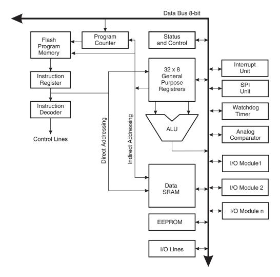
In order to maximize performance and parallelism, the Atmel<sup>®</sup> AVR uses a Harvard architecture – with separate memories and buses for program and data. Instructions in the program memory are executed with a single level pipelining. While one instruction is being executed, the next instruction is pre-fetched from the program memory. This concept enables instructions to be executed in every clock cycle. The program memory is In-System Reprogrammable Flash memory.
