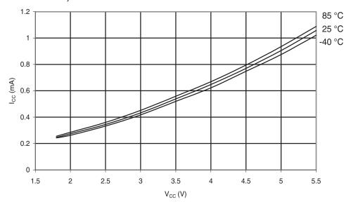
**Figure 6-232.** Atmel<sup>®</sup> ATmega168PA: Active Supply Current vs. V<sub>CC</sub> (Internal RC Oscillator, 8MHz)
