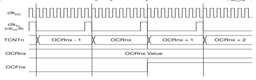
Figure 6-64 shows the setting of OCF2A and the clearing of TCNT2 in CTC mode.
