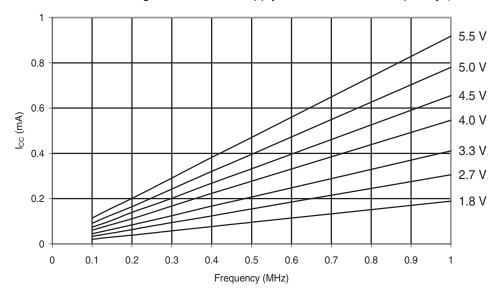
Figure 6-137. Atmel ATmega48PA: Active Supply Current vs. Frequency (1-20MHz)
