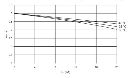
Figure 6-205. Atmel ATmega88PA: I/O Pin Output Voltage vs. Source Current ( $V_{CC} = 5V$ )
