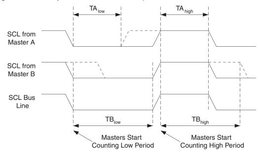
Figure 6-84. SCL Synchronization Between Multiple Masters
