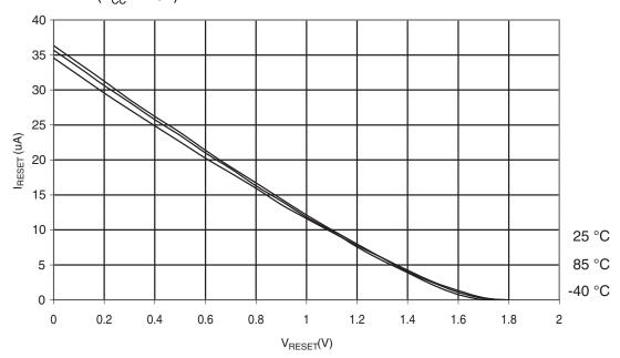
**Figure 6-292.** Atmel<sup>®</sup> ATmega328P: Reset Pull-up Resistor Current vs. Reset Pin Voltage  $(V_{CC} = 2.7V)$
