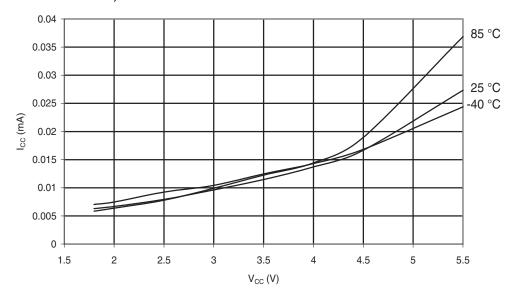
**Figure 6-236.** Atmel<sup>®</sup> ATmega168PA: Idle Supply Current vs. V<sub>CC</sub> (Internal RC Oscillator, 1MHz)
