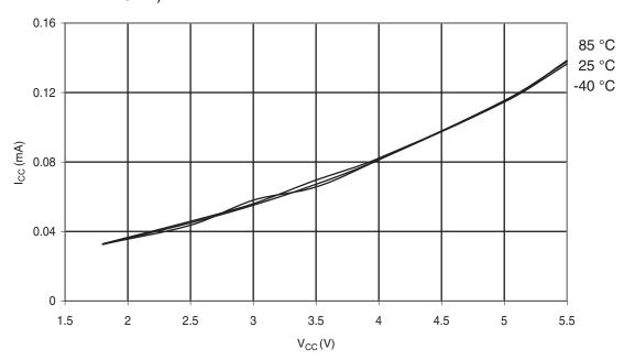
**Figure 6-277.** Atmel ATmega328P: Active Supply Current vs.  $V_{CC}$  (Internal RC Oscillator, 1MHz)
