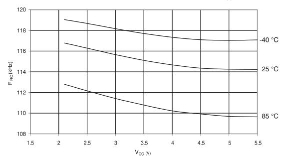
Figure 6-309. Atmel ATmega328P: Calibrated 8MHz RC Oscillator Frequency vs.  $V_{\rm CC}$
