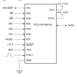
Note:  $V_{CC}$  - 0.3V < AV<sub>CC</sub> + 0.3V, however, AV<sub>CC</sub> should always be within 4.5 - 5.5V
