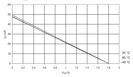
Figure 6-289. Atmel ATmega328P: I/O Pin Pull-up Resistor Current vs. Input Voltage  $(V_{CC}=2.7V)$
