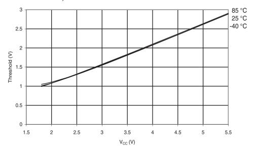
**Figure 6-253.** Atmel ATmega168PA: I/O Pin Input Threshold Voltage vs. V<sub>CC</sub> (V<sub>IL</sub>, I/O Pin read as '0')
