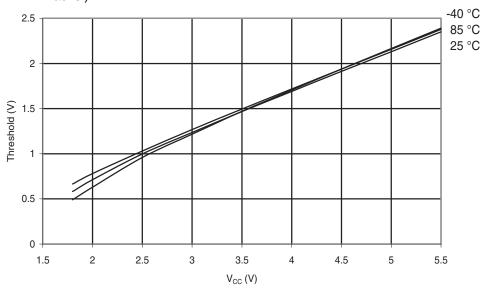
Figure 6-208. Atmel® ATmega88PA: I/O Pin Input Hysteresis vs. V<sub>CC</sub>
