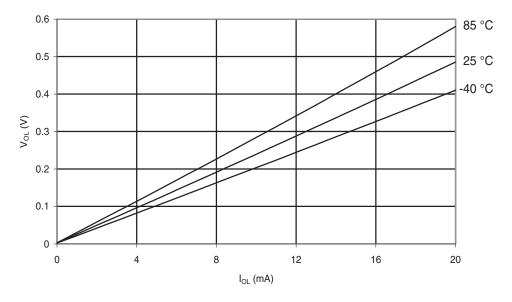
Figure 6-158. Atmel $^{\circledR}$  ATmega48PA: I/O Pin Output Voltage vs. Source Current( $V_{CC} = 3V$ )
