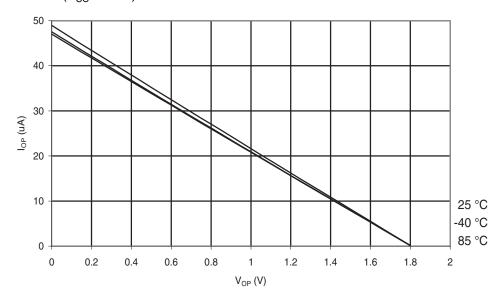
Figure 6-243. Atmel ATmega168PA: I/O Pin Pull-up Resistor Current vs. Input Voltage  $(V_{CC}=2.7V)$
