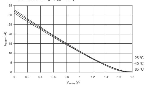
**Figure 6-154.** Atmel<sup>®</sup> ATmega48PA: Reset Pull-up Resistor Current vs. Reset Pin Voltage  $(V_{CC} = 2.7V)$
