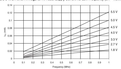
Figure 6-179. Atmel ATmega48PA: Reset Supply Current vs. Low Frequency (0.1 - 1.0MHz)
