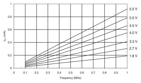
Figure 6-229. Atmel ATmega168PA: Active Supply Current vs. Frequency (1-20MHz)
