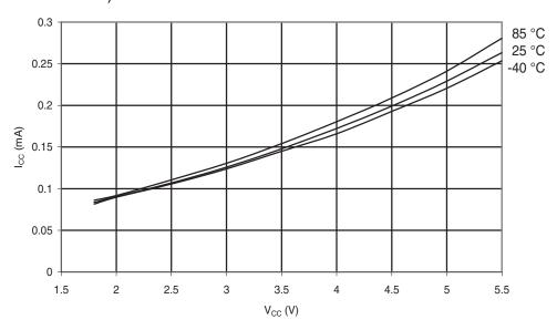
**Figure 6-237.** Atmel ATmega168PA: Idle Supply Current vs. Vcc (Internal RC Oscillator, 8MHz)
