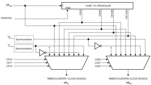
Figure 6-53. Prescaler for Timer/Counter0 and Timer/Counter1<sup>(1)</sup>
