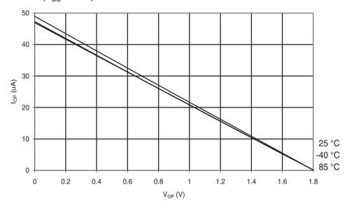
**Figure 6-197.** Atmel ATmega88PA: I/O Pin Pull-up Resistor Current vs. Input Voltage  $(V_{CC}=2.7V)$
