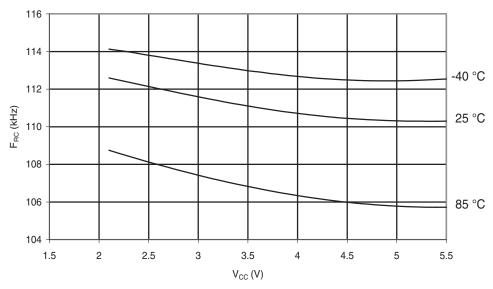
Figure 6-217. Atmel ATmega88PA: Calibrated 8 MHz RC Oscillator Frequency vs.  $V_{CC}$
