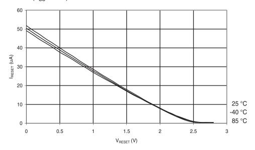
Figure 6-155. Atmel ATmega48PA: Reset Pull-up Resistor Current vs. Reset Pin Voltage  $(V_{CC} = 5V)$
