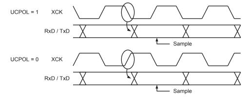
The UCPOLn bit UCRSC selects which XCKn clock edge is used for data sampling and which is used for data change. As Figure 6-72 shows, when UCPOLn is zero the data will be changed at rising XCKn edge and sampled at falling XCKn edge. If UCPOLn is set, the data will be changed at falling XCKn edge and sampled at rising XCKn edge.
