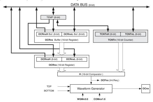
Figure 6-42. Output Compare Unit, Block Diagram
