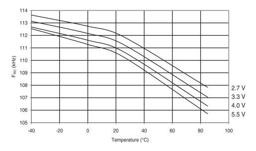
**Figure 6-216.** Atmel® ATmega88PA: Watchdog Oscillator Frequency vs.  $V_{CC}$
