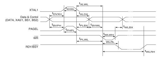
Figure 6-134. Parallel Programming Timing, Loading Sequence with Timing Requirements<sup>(1)</sup>
