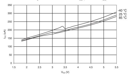
Figure 6-175. Atmel ATmega48PA: Analog Comparator Current vs.  $V_{CC}$
