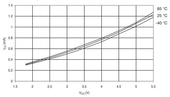
**Figure 6-278.** Atmel<sup>®</sup> ATmega328P: Active Supply Current vs. V<sub>CC</sub> (Internal RC Oscillator, 8MHz)
