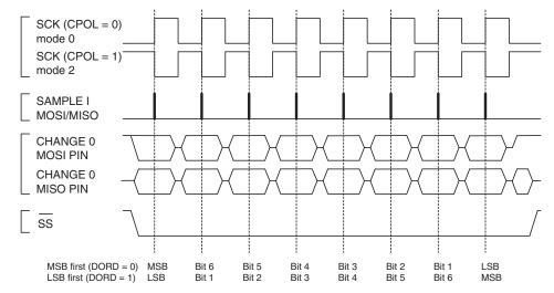
Figure 6-69. SPI Transfer Format with CPHA = 1
