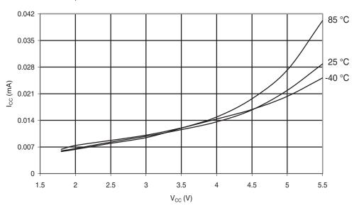
**Figure 6-144.** Atmel<sup>®</sup> ATmega48PA: Idle Supply Current vs. V<sub>CC</sub> (Internal RC Oscillator, 1MHz)
