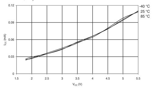
Figure 6-185. Atmel ATmega88PA: Active Supply Current vs.  $V_{CC}$  (Internal RC Oscillator, 1MHz)
