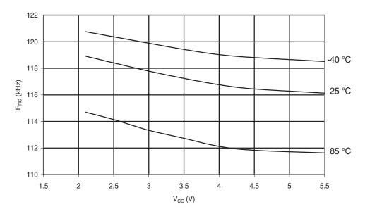
Figure 6-263. Atmel ATmega168PA: Calibrated 8MHz RC Oscillator Frequency vs.  $V_{CC}$
