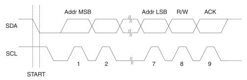
Figure 6-81. Address Packet Format
