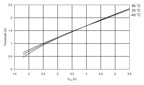
Figure 6-162. Atmel® ATmega48PA: I/O Pin Input Hysteresis vs. V<sub>CC</sub>
