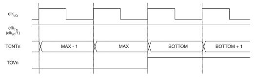
Figure 6-36 shows the same timing data, but with the prescaler enabled.
