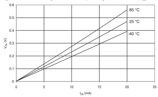
Figure 6-296. Atmel® ATmega328P: I/O Pin Output Voltage vs. Source Current (V<sub>CC</sub> = 3V)
