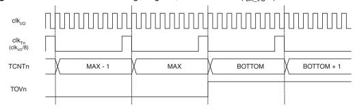
Figure 6-37 shows the setting of OCF0B in all modes and OCF0A in all modes except CTC mode and PWM mode, where OCR0A is TOP.
