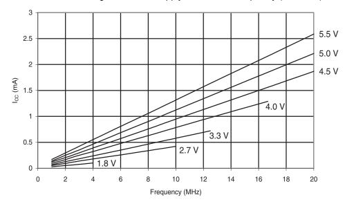
**Figure 6-143.** Atmel ATmega48PA: Idle Supply Current vs. V<sub>CC</sub> (Internal RC Oscillator, 128kHz)
