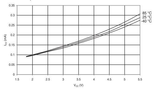
**Figure 6-145.** Atmel ATmega48PA: Idle Supply Current vs. Vcc (Internal RC Oscillator, 8MHz)
