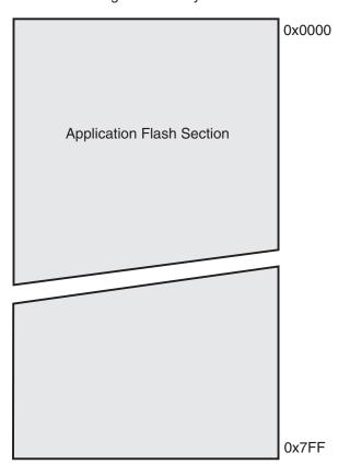
**Figure 6-8.** Program Memory Map Atmel ATmega88PA, ATmega168PA and ATmega328P Program Memory
