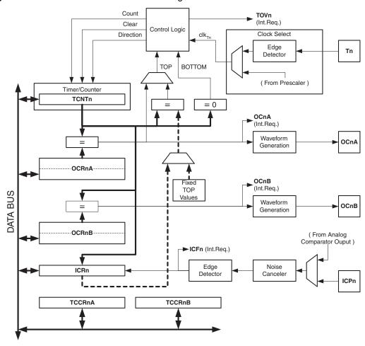
Figure 6-39. 16-bit Timer/Counter Block Diagram<sup>(1)</sup>
