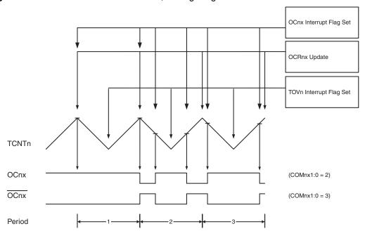
The Timer/Counter Overflow Flag (TOV0) is set each time the counter reaches BOTTOM. The Interrupt Flag can be used to generate an interrupt each time the counter reaches the BOTTOM value.
