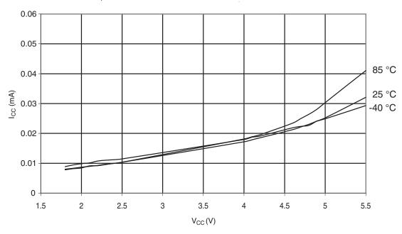
**Figure 6-282.** Atmel $^{\circledR}$  ATmega328P: Idle Supply Current vs.  $V_{CC}$  (Internal RC Oscillator, 1MHz)
