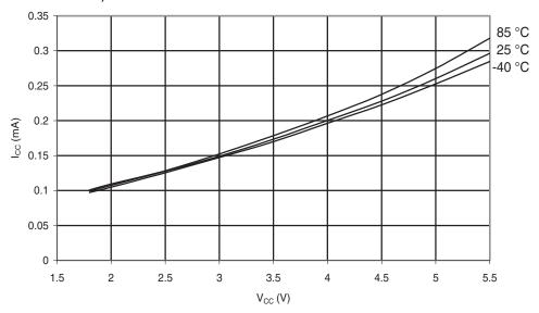
**Figure 6-191.** Atmel ATmega88PA: Idle Supply Current vs. Vcc (Internal RC Oscillator, 8MHz)
