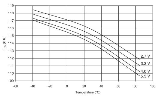
**Figure 6-308.** Atmel<sup>®</sup> ATmega328P: Watchdog Oscillator Frequency vs.  $V_{CC}$
