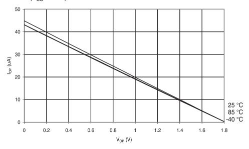
**Figure 6-151.** Atmel ATmega48PA: I/O Pin Pull-up Resistor Current vs. Input Voltage  $(V_{CC}=2.7\ V)$
