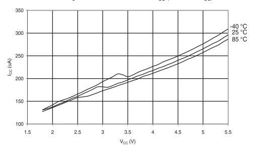
Figure 6-267. Atmel ATmega168PA: Analog Comparator Current vs.  $V_{CC}$
