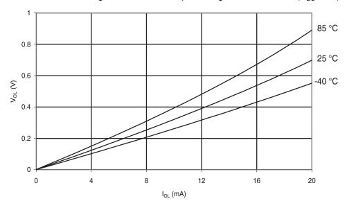
Figure 6-157. Atmel ATmega48PA: I/O Pin Output Voltage vs. Sink  $Current(V_{CC} = 5V)$
