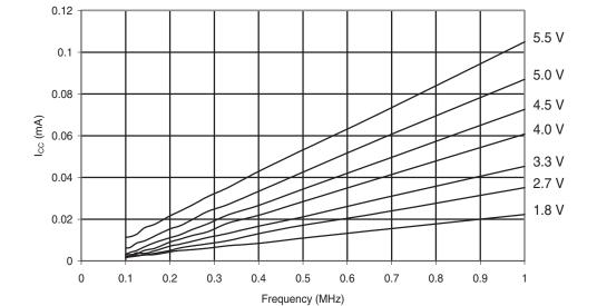
Figure 6-225. Atmel ATmega88PA: Reset Supply Current vs. Low Frequency (0.1 - 1.0MHz)
