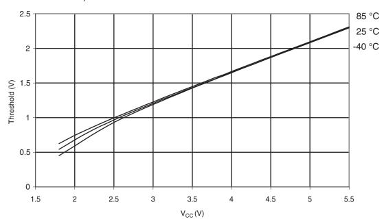
Figure 6-300. Atmel $^{\tiny{(8)}}$  ATmega328P: I/O Pin Input Hysteresis vs.  $V_{\tiny{CC}}$
