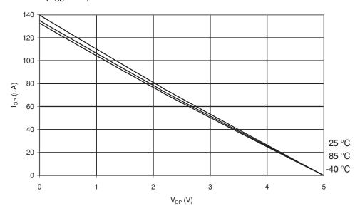
**Figure 6-199.** Atmel ATmega88PA: Reset Pull-up Resistor Current vs. Reset Pin Voltage  $(V_{CC}=1.8V)$
