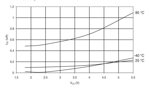
**Figure 6-147.** Atmel ATmega48PA: Power-Down Supply Current vs.  $V_{CC}$  (Watchdog Timer Enabled)
