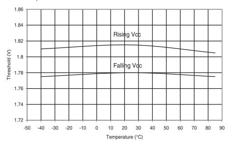
Figure 6-259. Atmel ATmega168PA: BOD Thresholds vs. Temperature (BODLEVEL is 2.7V)
