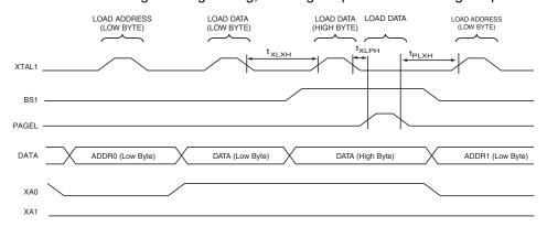
Note: 1. The timing requirements shown in Figure 6-133 (i.e., t<sub>DVXH</sub>, t<sub>XHXL</sub>, and t<sub>XLDX</sub>) also apply to loading operation.
