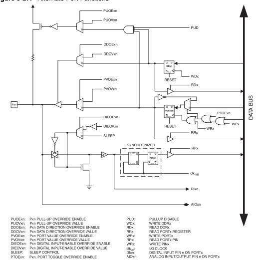
Note: 1. WRx, WPx, WDx, RRx, RPx, and RDx are common to all pins within the same port. clk<sub>I/O</sub>, SLEEP, and PUD are common to all ports. All other signals are unique for each pin.
