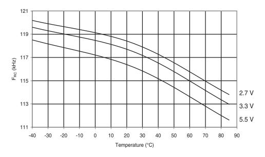
Figure 6-262. Atmel® ATmega168PA: Watchdog Oscillator Frequency vs. V<sub>CC</sub>
