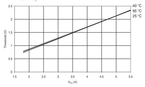
**Figure 6-257.** Atmel ATmega168PA: Reset Pin Input Hysteresis vs.  $V_{CC}$
