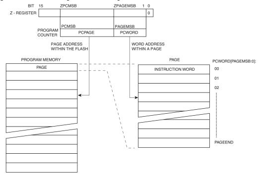
Figure 6-115. Addressing the Flash During SPM<sup>(1)</sup>
