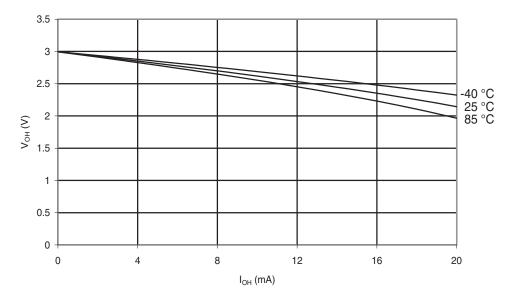
Figure 6-159. Atmel ATmega48PA: I/O Pin Output Voltage vs. Source Current(V<sub>CC</sub> = 5V)
