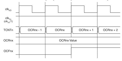
Figure 6-49 shows the same timing data, but with the prescaler enabled.
