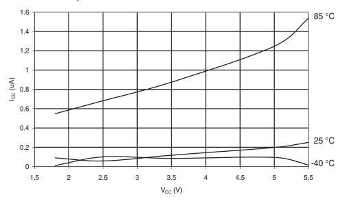
**Figure 6-193.** Atmel ATmega88PA: Power-Down Supply Current vs.  $V_{CC}$  (Watchdog Timer Enabled)
