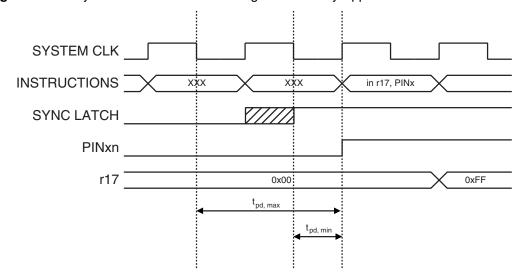
Figure 6-25. Synchronization when Reading an Externally Applied Pin value
