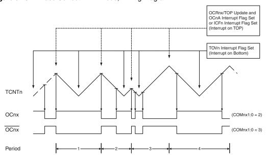
The Timer/Counter Overflow Flag (TOV1) is set each time the counter reaches BOTTOM. When either OCR1A or ICR1 is used for defining the TOP value, the OC1A or ICF1 Flag is set accordingly at the same timer clock cycle as the OCR1x Registers are updated with the double buffer value (at TOP). The Interrupt Flags can be used to generate an interrupt each time the counter reaches the TOP or BOTTOM value.
