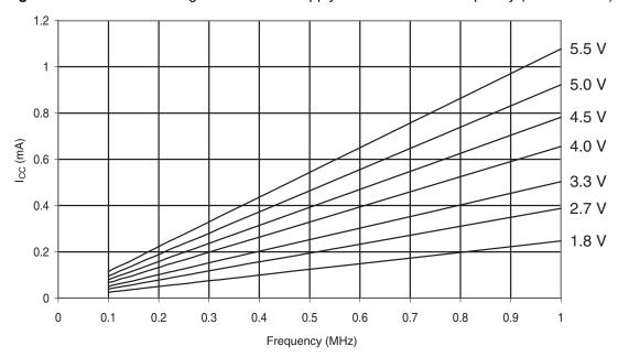
Figure 6-275. Atmel ATmega328P: Active Supply Current vs. Frequency (1 - 20MHz)
