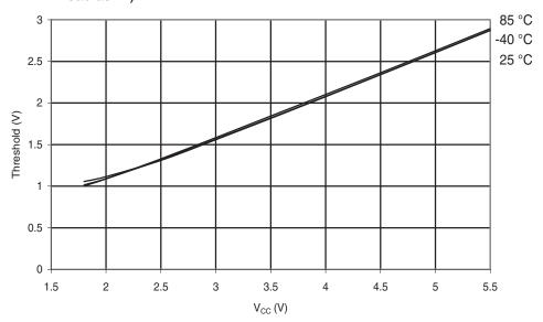
**Figure 6-207.** Atmel ATmega88PA: I/O Pin Input Threshold Voltage vs.  $V_{CC}$  ( $V_{/L}$ , I/O Pin read as '0')
