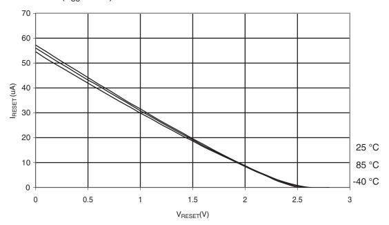
Figure 6-293. Atmel ATmega328P: Reset Pull-up Resistor Current vs. Reset Pin Voltage  $(V_{CC} = 5V)$
