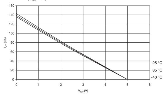
Figure 6-291. Atmel ATmega328P: Reset Pull-up Resistor Current vs. Reset Pin Voltage  $(V_{CC}=1.8V)$
