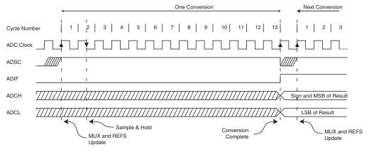
Figure 6-106. ADC Timing Diagram, Auto Triggered Conversion
