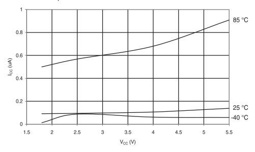
**Figure 6-239.** Atmel ATmega168PA: Power-Down Supply Current vs.  $V_{CC}$  (Watchdog Timer Enabled)
