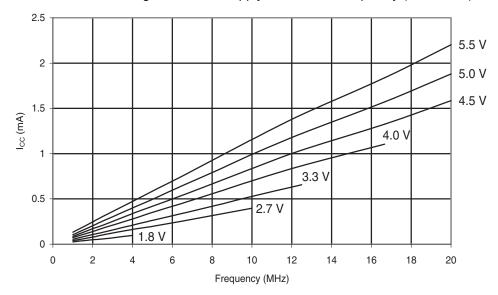
**Figure 6-189.** Atmel ATmega88PA: Idle Supply Current vs.  $V_{CC}$  (Internal RC Oscillator, 128kHz)
