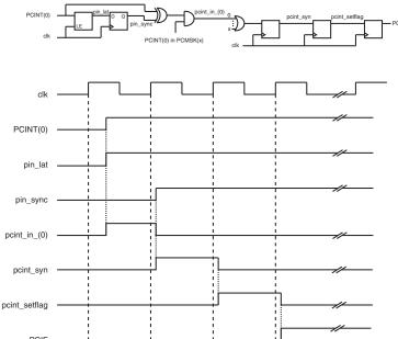
Figure 6-22. Timing of pin change interrupts
