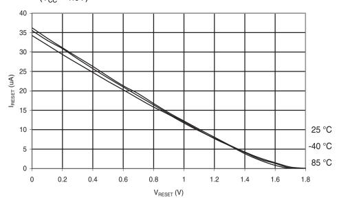
**Figure 6-200.** Atmel<sup>®</sup> ATmega88PA: Reset Pull-up Resistor Current vs. Reset Pin Voltage  $(V_{CC} = 2.7V)$
