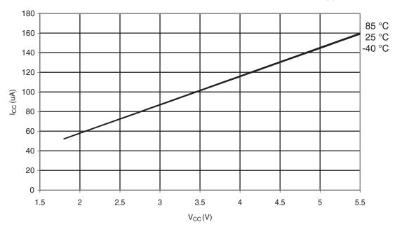
Figure 6-315. Atmel ATmega328P: Brownout Detector Current vs.  $V_{CC}$
