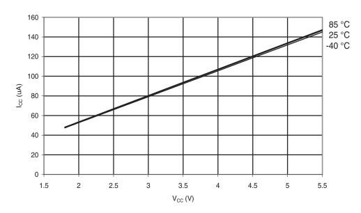
Figure 6-177. Atmel ATmega48PA: Brownout Detector Current vs.  $V_{CC}$
