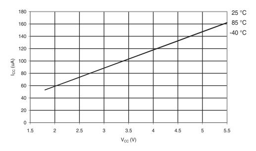
Figure 6-269. Atmel ATmega168PA: Brownout Detector Current vs.  $V_{CC}$
