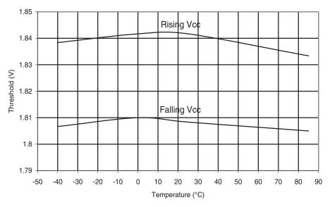
Figure 6-167. Atmel ATmega48PA: BOD Thresholds vs. Temperature (BODLEVEL is 2.7V)
