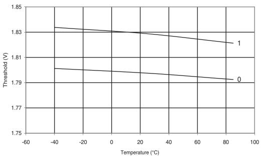
Figure 6-305. Atmel ATmega328P: BOD Thresholds vs. Temperature (BODLEVEL is 2.7V)
