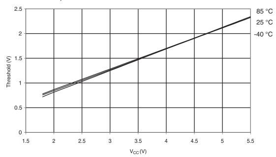
Figure 6-303. Atmel ATmega328P: Reset Pin Input Hysteresis vs.  $V_{\rm CC}$
