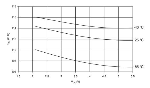
Figure 6-171. Atmel ATmega48PA: Calibrated 8 MHz RC Oscillator Frequency vs.  $V_{\rm CC}$
