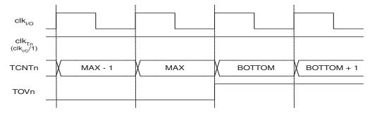
Figure 6-62 shows the same timing data, but with the prescaler enabled.
