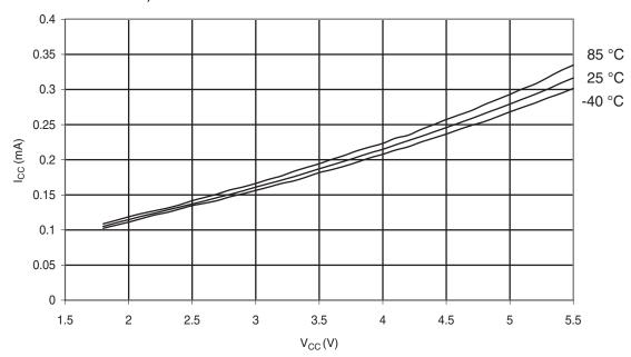
Figure 6-283. Atmel ATmega328P: Idle Supply Current vs. Vcc (Internal RC Oscillator, 8MHz)
