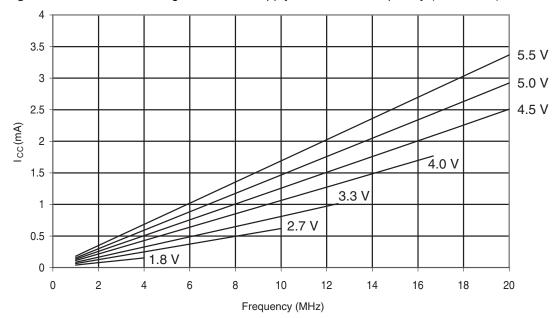
**Figure 6-281.** Atmel ATmega328P: Idle Supply Current vs. V<sub>CC</sub> (Internal RC Oscillator, 128kHz)
