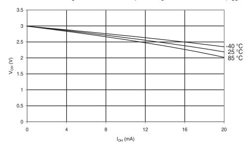
Figure 6-251. Atmel ATmega168PA: I/O Pin Output Voltage vs. Source  $Current(V_{CC} = 5V)$
