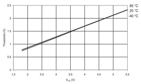
Figure 6-211. Atmel ATmega88PA: Reset Pin Input Hysteresis vs.  $V_{\rm CC}$
