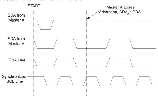
Figure 6-85. Arbitration Between Two Masters
