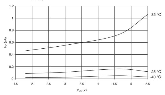
$\textbf{Figure 6-285.} \ \, \textbf{ATmega328P: Power-Down Supply Current vs. V}_{\text{CC}} \ \, \textbf{(Watchdog Timer Enabled)}$
