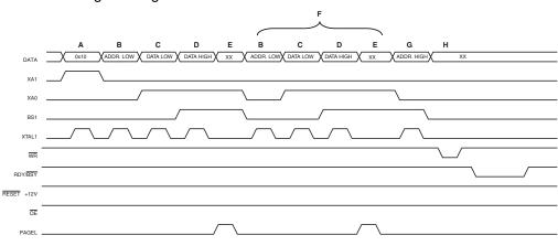
Figure 6-121. Programming the Flash Waveforms<sup>(1)</sup>
