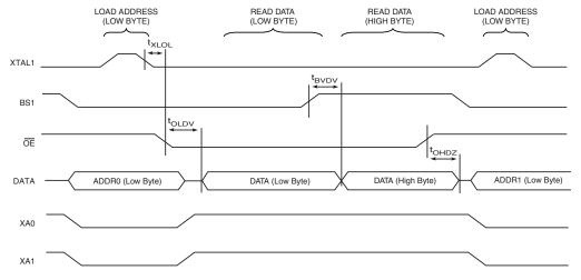
Note: 1. The timing requirements shown in Figure 6-133 (i.e., t<sub>DVXH</sub>, t<sub>XHXL</sub>, and t<sub>XLDX</sub>) also apply to reading operation.
