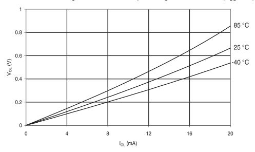
Figure 6-249. Atmel ATmega168PA: I/O Pin Output Voltage vs. Sink Current( $V_{CC} = 5V$ )
