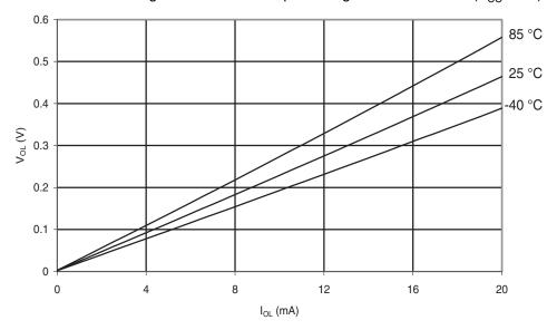
Figure 6-204. Atmel® ATmega88PA: I/O Pin Output Voltage vs. Source Current (V<sub>CC</sub> = 3V)
