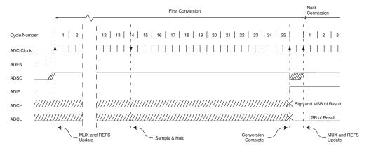
Figure 6-105. ADC Timing Diagram, Single Conversion
