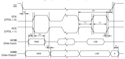
Figure 6-131. SPI Interface Timing Requirements (Slave Mode)
