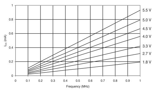
Figure 6-183. Atmel ATmega88PA: Active Supply Current vs. Frequency (1 - 20MHz)
