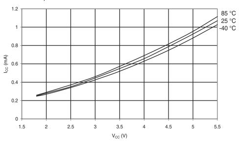
**Figure 6-140.** Atmel® ATmega48PA: Active Supply Current vs. V<sub>CC</sub> (Internal RC Oscillator, 8MHz)
