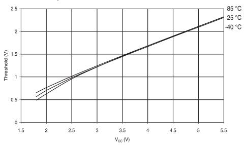
Figure 6-254. Atmel $^{\tiny{(8)}}$  ATmega168PA: I/O Pin Input Hysteresis vs.  $V_{\tiny{CC}}$
