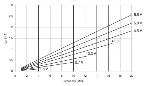
**Figure 6-235.** Atmel $^{\otimes}$  ATmega168PA: dle Supply Current vs.  $V_{CC}$  (Internal RC Oscillator, 128kHz)
