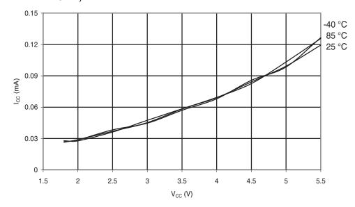
**Figure 6-231.** Atmel ATmega168PA: Active Supply Current vs.  $V_{CC}$  (Internal RC Oscillator, 1MHz)
