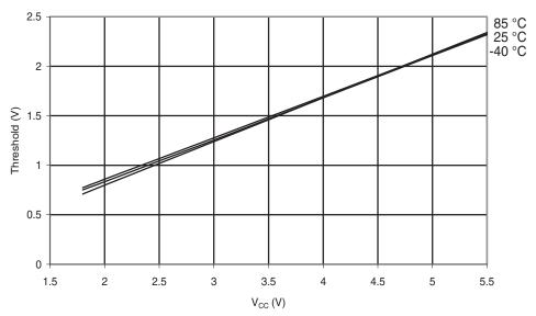
Figure 6-165. Atmel ATmega48PA: Reset Pin Input Hysteresis vs.  $V_{\rm CC}$
