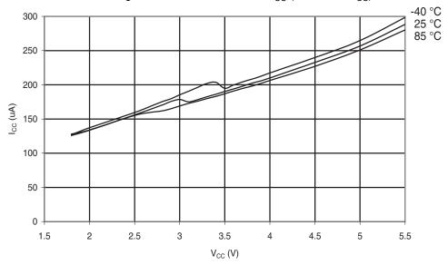
Figure 6-221. Atmel ATmega88PA: Analog Comparator Current vs.  $V_{CC}$
