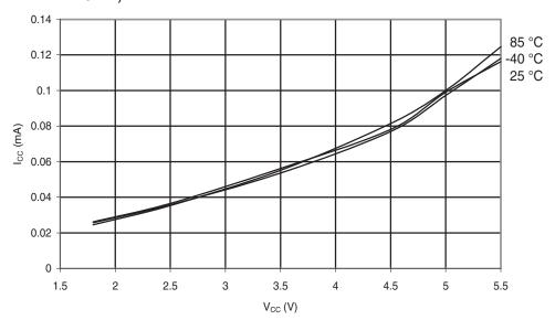
**Figure 6-139.** Atmel ATmega48PA: Active Supply Current vs.  $V_{CC}$  (Internal RC Oscillator, 1MHz)
