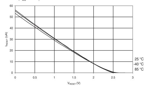
Figure 6-247. Atmel ATmega168PA: Reset Pull-up Resistor Current vs. Reset Pin Voltage  $(V_{CC}=5V)$
